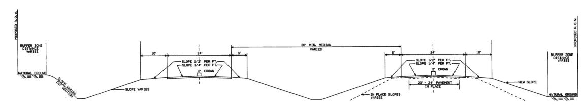
NEW CONSTRUCTION REQ'D 24' BITUMINOUS CONCRETE PAVEMENT
